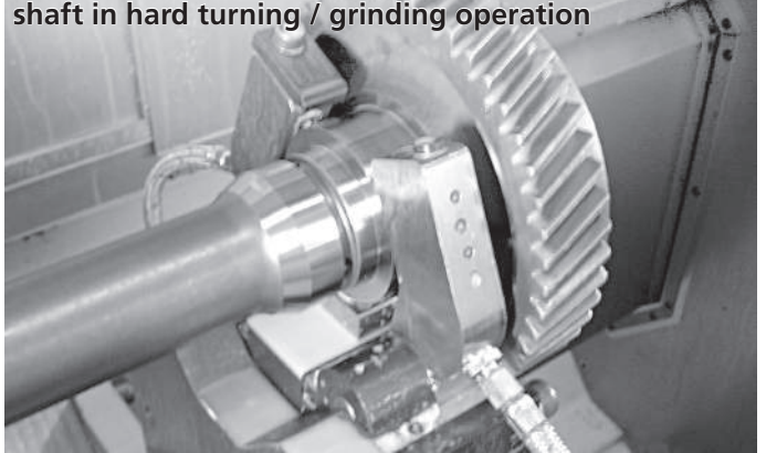
Steady Rest clamping aircraft shaft
